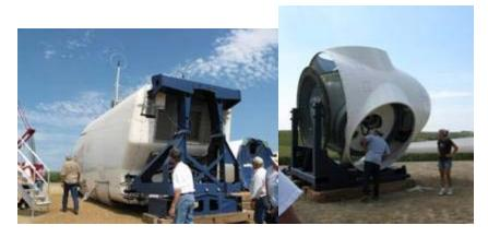
This nacelle is the size of a bus! It will be placed at the top of the tower. This holds the generator and has working area. The hub will be attached to the nacelle and placed at the top of the tower and have the blades attached to it.
